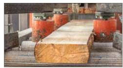
Large throat capacity (2.2'/26.7" wide) to process large-dimensioned and heavy flitches, cants or blocks into precisely sawn product.
