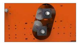
With dual arbors, smaller diameter / thinner kerf saws can be used to boost recovery. Collared saw spacers and strobe saws simplify saw maintenance.
